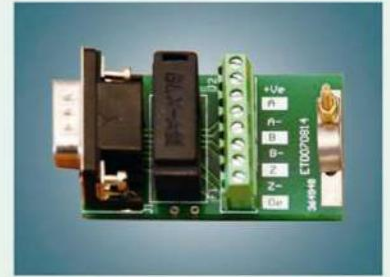
ENCODER CONNECTION BOARD
